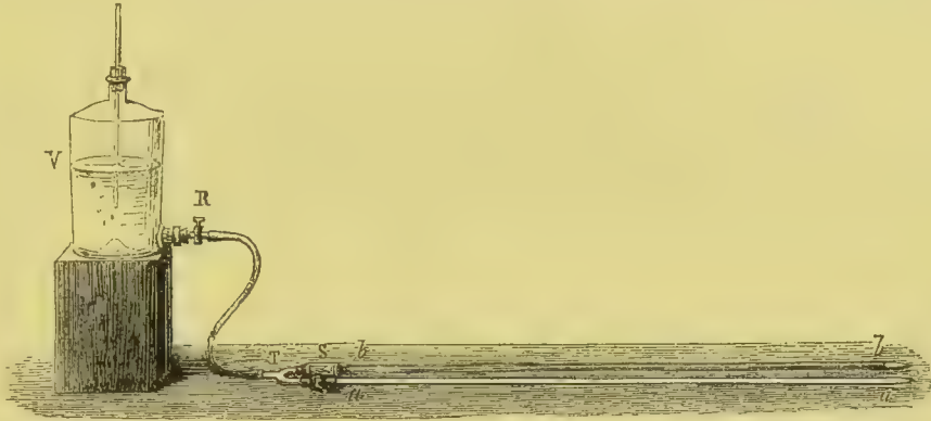
FIG. 21.—Apparatus for showing the action of the elasticity of the arteries. (Marey.)
